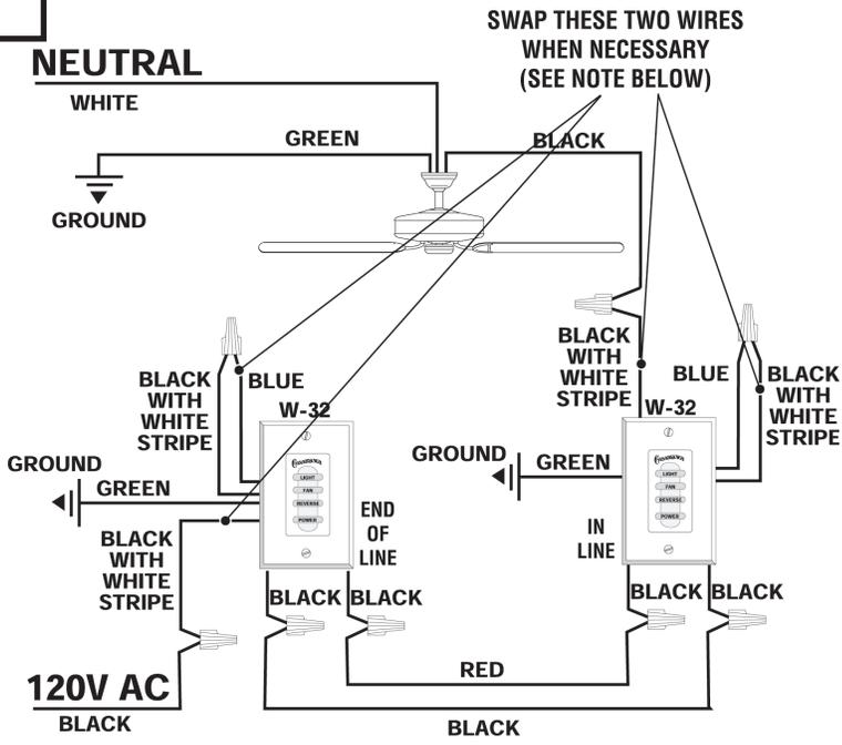
**NOTE:** If wall control operation is reversed (fan switch controls lights and light switch controls fan) turn off the power at the breaker or fuse panel, then swap the two W-32 black/white stripe wires.
